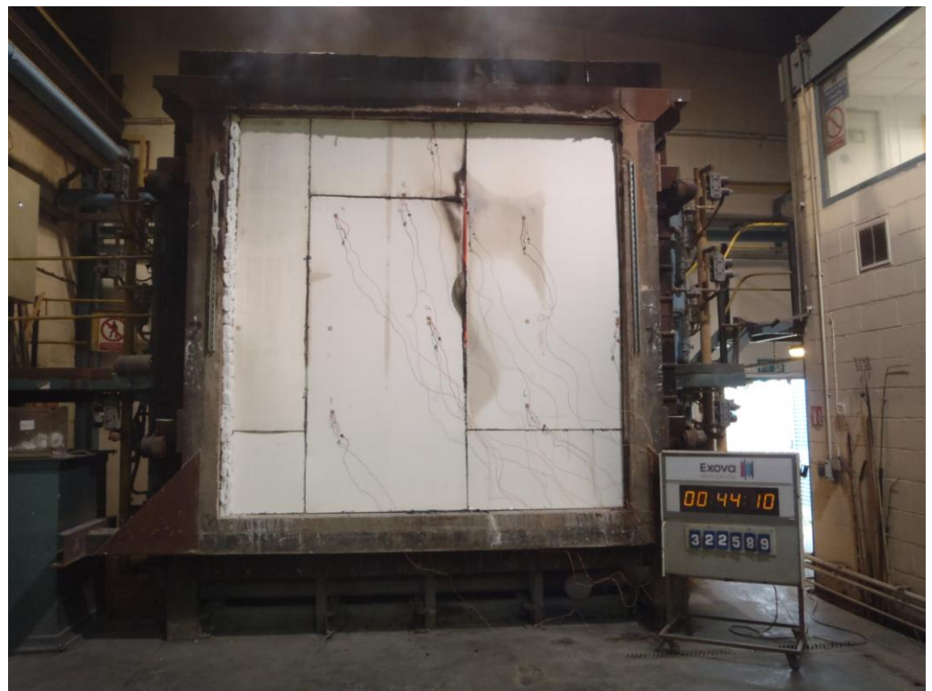
The unexposed face of the test construction after a test duration of 44 minutes
