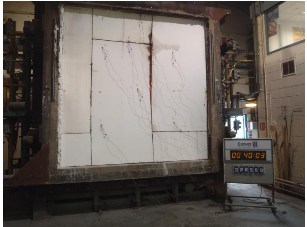
The unexposed face of the test construction after a test duration of 40 minutes
