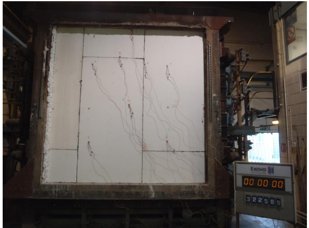
The unexposed face of the test construction prior to testing
