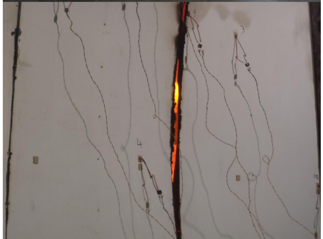
The unexposed face of the test construction after a test duration of 37 minutes
