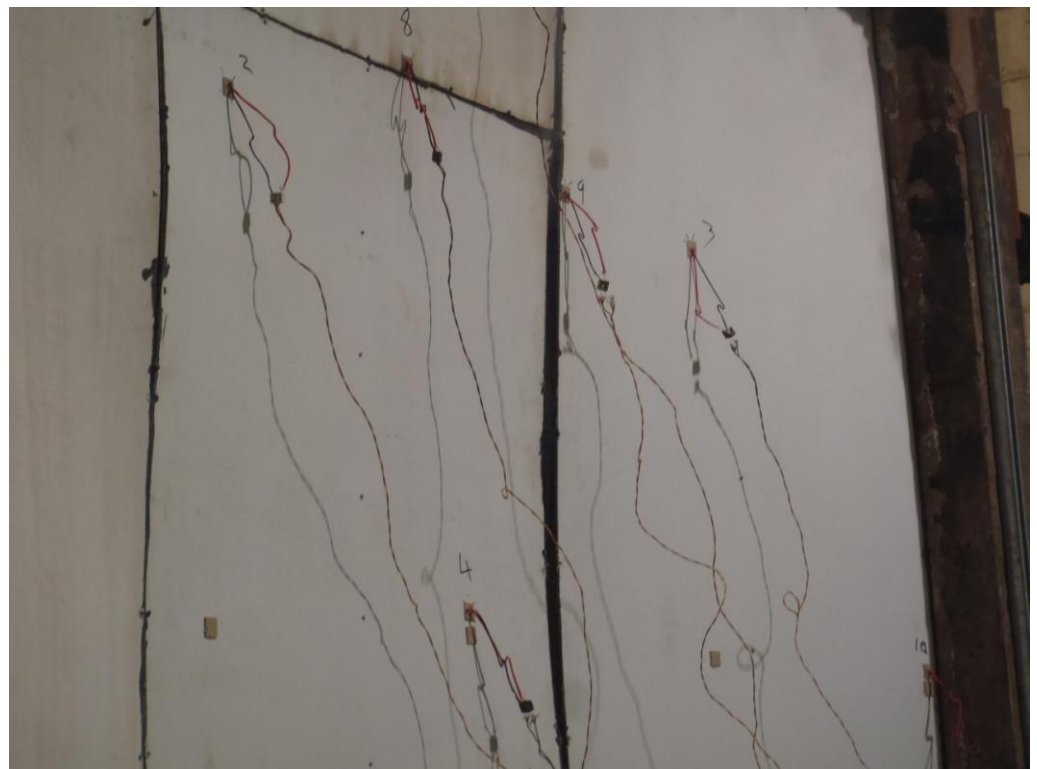
The unexposed face of the test construction after a test duration of 20 minutes
