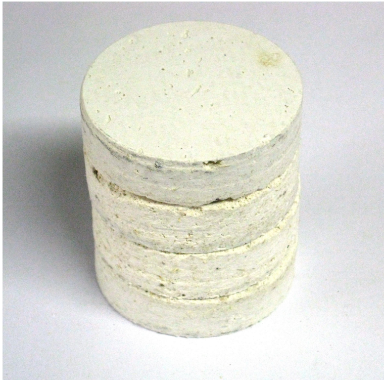
Figure A.1 Photograph of an EN ISO 1182 test specimen as received
